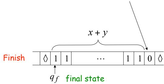
Turing machine for function  $f(x, y) = x + y$
