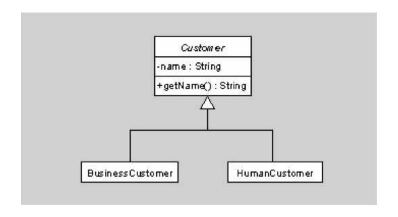
Generalization by moving common behavior to a superclass.
