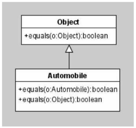
The Automobile class does not inherit the Object class' equals method. Instead, it overrides that method.
