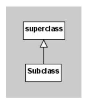
The UML notation for subclass and superclass.
