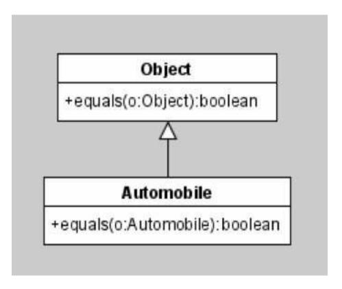
The Automobile class has two equals methods, one inherited and one defined in Automobile.
