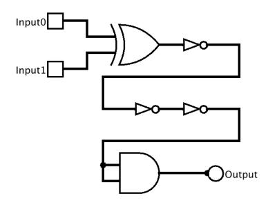
2) Which output signal is asserted for all possible values for Input1 (most significant) and Input0 (least significant) in binary order 00, 01, 10, 11?
