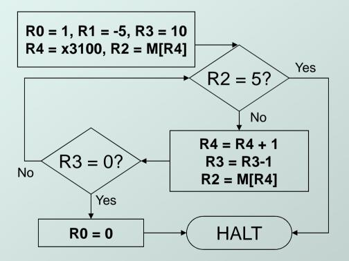
x3000 010100000100000 x3001 000100000100001 x3002 0101001001100000 x3003 0001001001111011 x3004 0101011011100000 x3005 0001011011101010 x3006 0010100000001001 x3007 011001010000000 x3008 0001010010000001 x3009 0000010000000101 x300A 0001100100100001 x300B 000101101111111 x300C 011001010000000 x300D 000001111111010 x300E 010100000100000 x300F 1111000000100101 x3010 001100010000000
