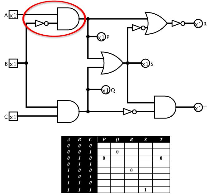
Now apply De-Morgan's laws to change the part of the circuit that is in the red oval, design the modified circuit in Logisim and turn in the schematic, and its new truth table.
