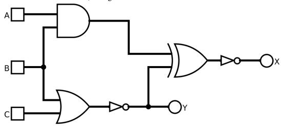
2) Find truth table values by manually toggling the input values and examining the output values. This is done in Logisim by selecting the hand icon and then clicking on each input. Fill in the rest of the truth table for the circuit manually:
