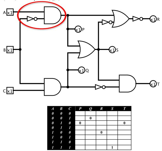
Now apply De-Morgan's laws to change the part of the circuit that is in the red oval, design the modified circuit in Logisim and turn in the schematic (print it out and attach the sheet, and its new truth table.
