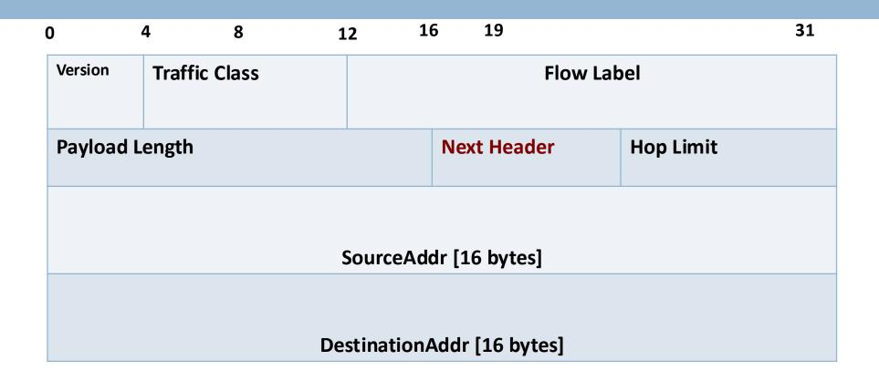
IPv6 Packet Header is fixed at 40 bytes ... So there is no Header Length
