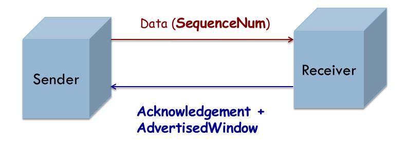
Each byte of data has a sequence number SequenceNum contains sequence number for first byte of data in segment
