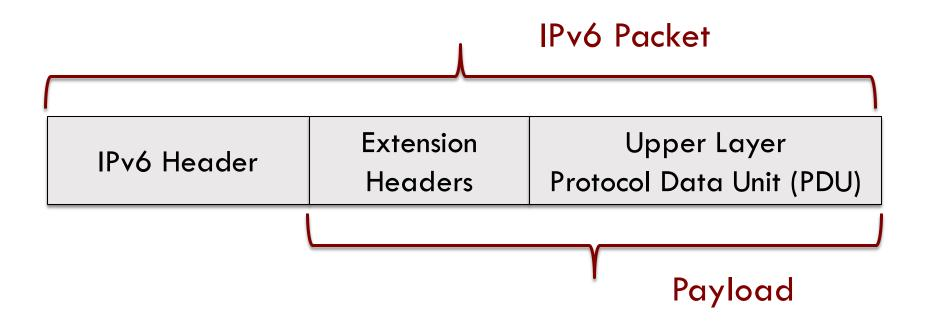
PDU typically contains an upper layer protocol header and its payload. For e.g.: a TCP segment, UDP Datagram, or an ICMPv6 message
